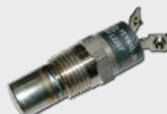
HEAVY DUTY TEMP SWITCH 104°C N/C THREAD: 3/8 NPT PART NO. 1765
