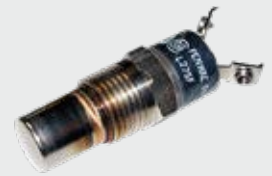
HEAVY DUTY TEMP SWITCH 135°C N/C THREAD: 3/8 NPT PART NO. 1768
