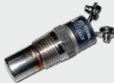
HEAVY DUTY TEMP SWITCH 100°C N/C THREAD: 3/8 NPT PART NO. 1764
